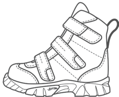
Waterproof boot with warm felt lining, Vibram sole and bellows tongue
